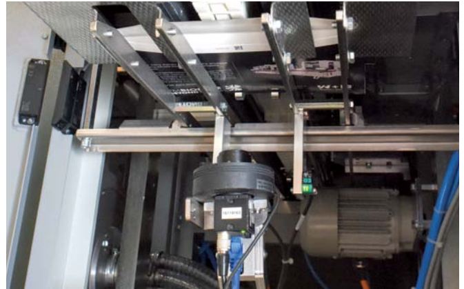
Camera reading for Code on the envelope
